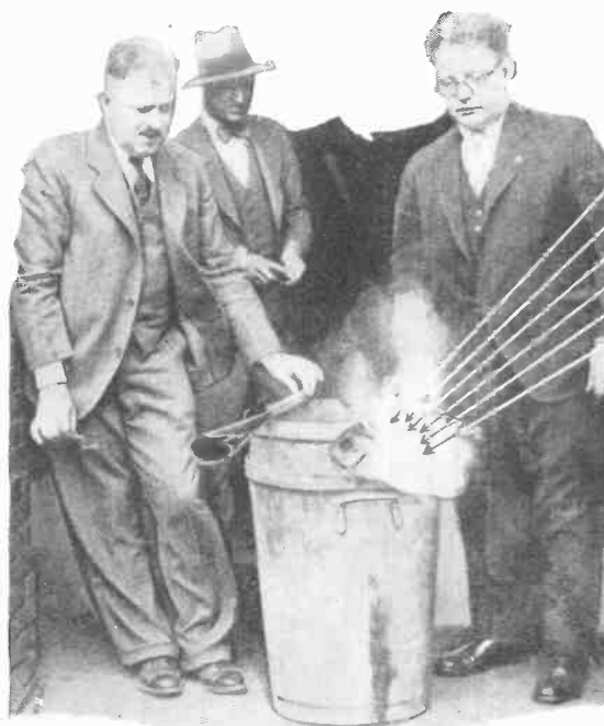
Showing the difference between slow-burning and regular X-ray film. Note blaze at right giving off the gases.
