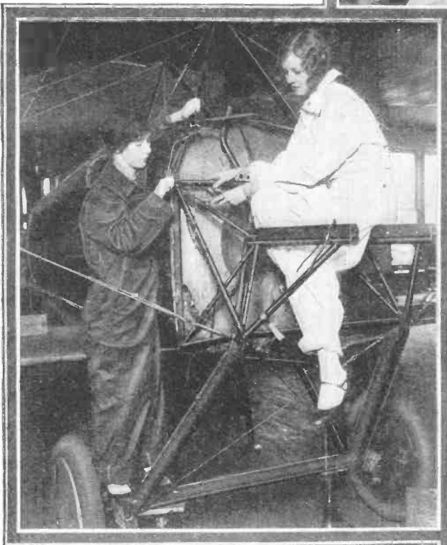
The above photograph shows Miss Betty Sessur and Miss Mildred Miller working on the front of a plane preparatory to installing the engine. At the right four of the students are shown repairing one of the airplane engines in conjunction with their aviation course. The engine is completely taken apart and then assembled by the students for practice and experience.
