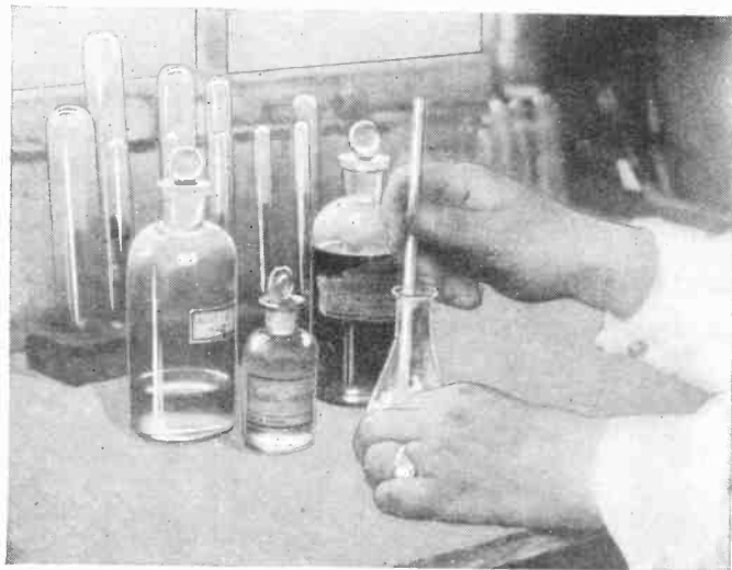
In order to make cellulose acetate, some cotton is pressed into a flask and 20 c.c. of acetic acid, 6 c.c. of acetic anhydride and a drop or two of sulphuric acid are added.
